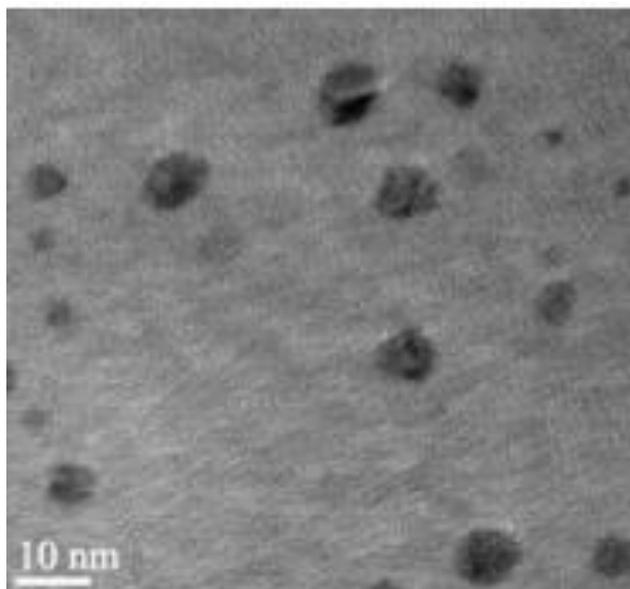
Figure 5: TEM image of nanoparticles
