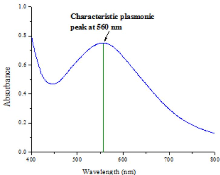
Figure 3: UV-Vis curve recorded after 24 Hrs of incubation
