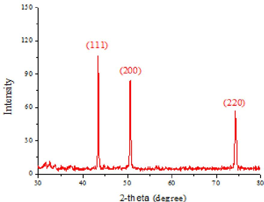
Figure 4: XRD graph of extract-mediated Cu nanoparticles
