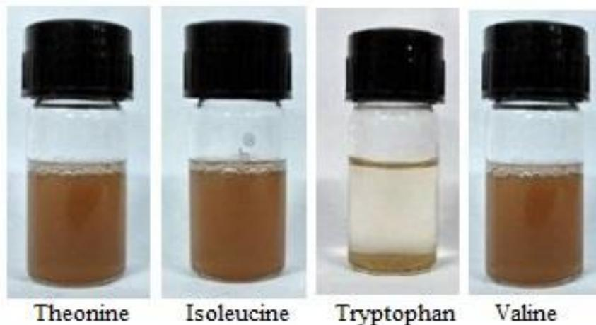
Figure 6. Colorimetric detection of tryptophan by suspension of nano-copper
